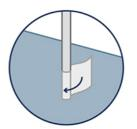
Make sure that any penetration up through the floor also gets ISO around it. (e.g. water pipes, drain pipes, and any other object protruding from the floor)
