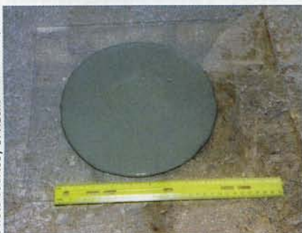
Monitoring the water content of gypsum concrete floor underlayments.
