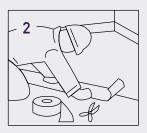
Seams between sound mat rolls are adhered with tape.
