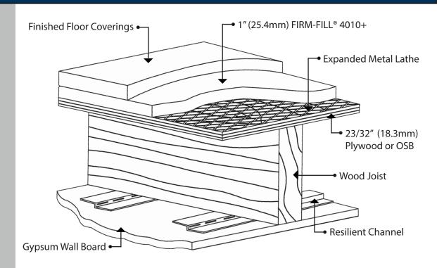
When installing FIRM-FILL® 4010+ over wood substrate, reinforcement is needed. Both Clark Dietrich's® and CEMCO's® expanded metal lath create addiquate reinformcement over wood substrate. Its carefully formed diamond keys allow for proper embedment and keying of the scratch coat on all types of substrates.
