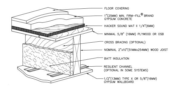
When installed over Nominal Wood Joist, 1.25" (32mm) FIRM-FILL® Brand Gypsum Concrete and Hacker Sound Mat II achieve excellent fire and sound ratings, while providing a superior crackresistant surface surface for the installation of finished floor coverings.
