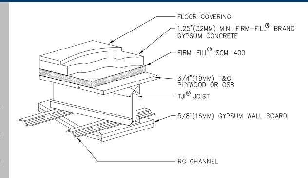
When installed over an I-Joist, 1.25" (32mm) FIRM-FILL® Brand Gypsum Concrete and 3/8" (10mm) FIRM-FILL® SCM-400 achieve excellent fire and sound ratings while providing a superior crack-resistant surface for the installation of finished floor coverings.
