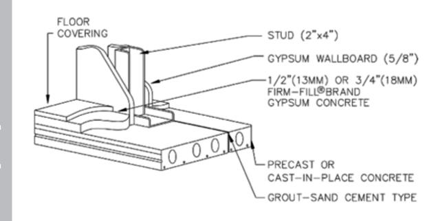
When installed at 1/2" (13mm) or 3/4" (19)mm over precast concrete, FIRM-FILL® Brand Gypsum Concrete achieves excellent fire and sound ratings while providing a superior crack-resistant surface for the installation of finished floor coverings.
