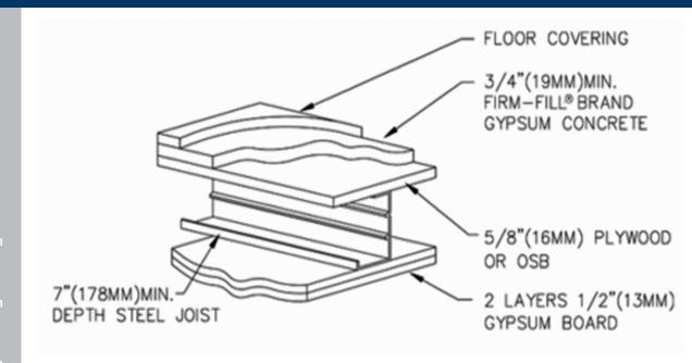
When installed at 3/4" over steel truss with plywood, FIRM-FILL® Brand Gypsum Concrete achieves excellent fire and sound ratings while providing a superior crack-resistant surface for the installation of finished floor coverings.
